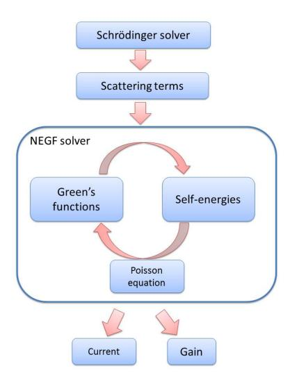
In the beginning of the calculation, the single-band effective mass Schrödinger equation is solved in real space. The energy levels (i.e. minibands) are selected up to an energy cut-off which is specified
