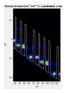
Then, the main part of the calculation consists in the self-consistent NEGF solver. Starting from an initial guess of the Green's functions, the self-energies are calculated. The Green's functions are then calculated iteratively. Simultaneously, the mean-field electrostatic potential is calculated self-consistently (Poisson's equation). Such iterations are made until convergence is reached for the Green's functions as well as for the calculated current.
